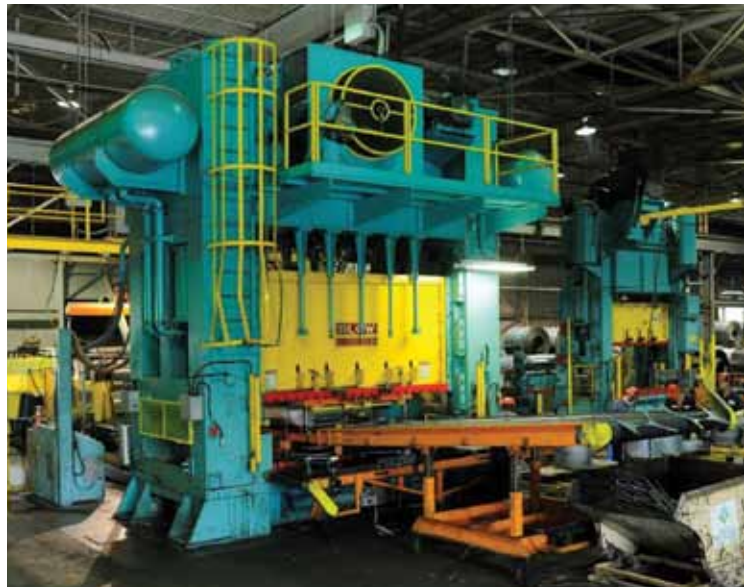
Heidtman’s Toledo Blank facility offers first-operation blanking for customers in the appliance, HVAC, tank and automotive industries. Shown: a 1,200-ton press at the Toledo plant. (Photo courtesy Heidtman)
